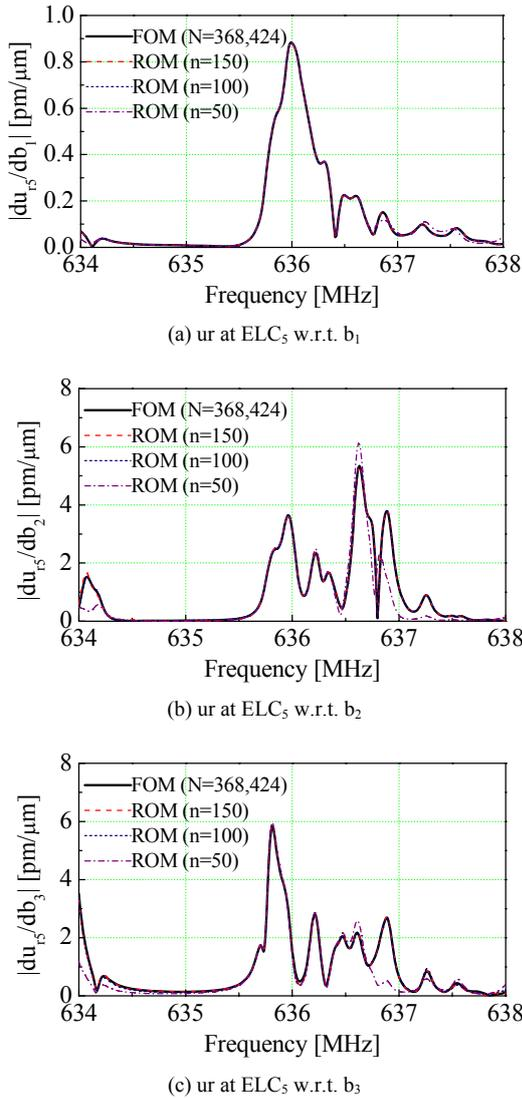
Fig. 15. Design sensitivities of the frequency responses at ELC<sub>5</sub> according to the order of reduced models.
