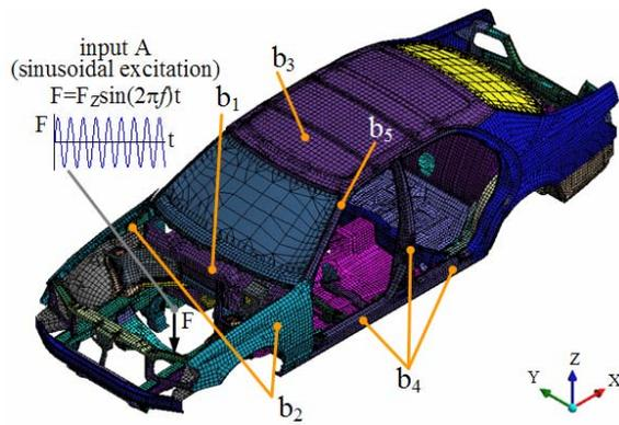
Fig. 1. The finite element model of a car body.
