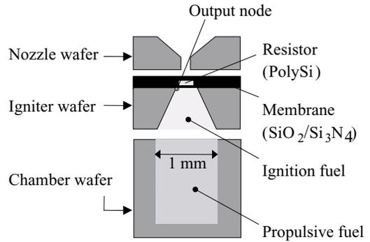
Fig. 1 Microthruster structure.
