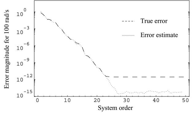
Fig. 4 Error estimate for  $\omega = 10^2 \text{ rad/s}$ .
