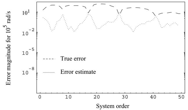
Fig. 6 Error estimate for  $\omega = 10^5 \text{ rad/s}$ .
