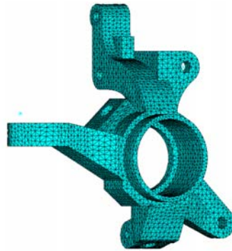
Fig. 3 FE mesh for the knuckle
