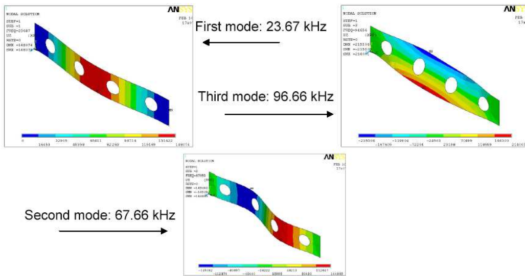
Figure 2: The modal analysis for the first three vibrational modes of the switch. The modal analysis was performed with the commercially available FE-code ANSYS. The mode shape functions are color encoded.
