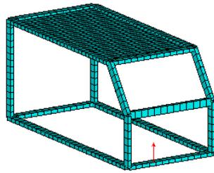
Figure 2(a): Structural FE model
