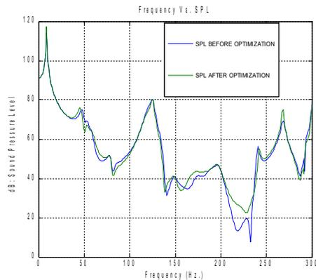
*Figure: 6: Sound pressure levels before and after optimization.*
