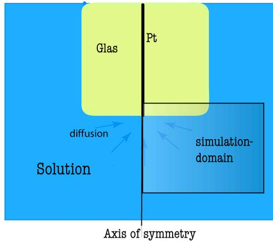
Fig. 3. The layout of electrochemistry simulation.
