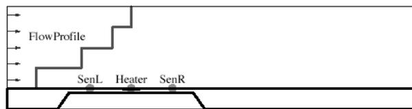
Fig. 5. Model of the anemometer. The flow enters from the left. A heater is surrounded by two thermosensors.
