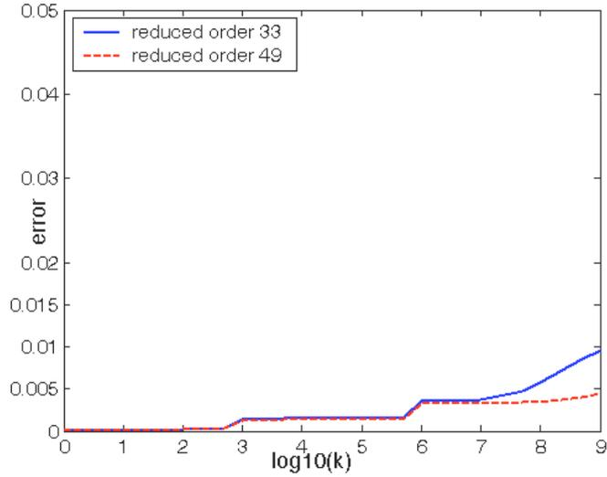
Fig. 2. The error of transient simulation for a reduced model as a function of the film coefficient. Note that the film coefficient changes by nine orders of magnitude.
