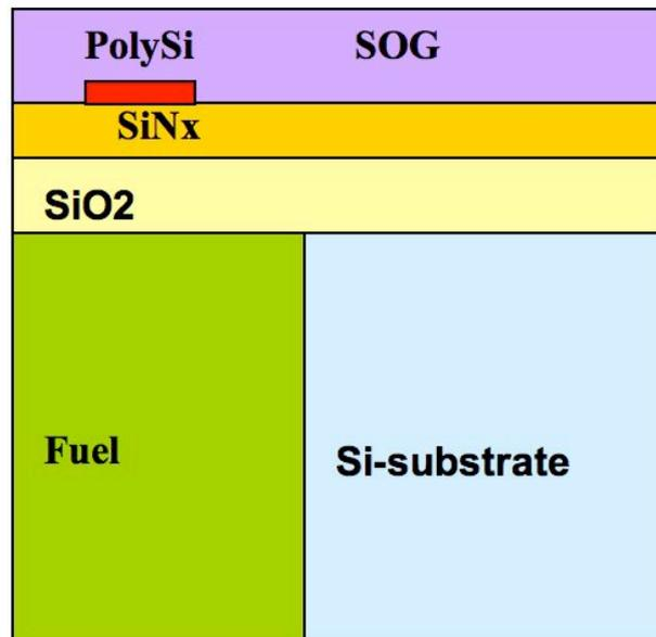
Fig. 1. A 2D-axisymmetrical model of the microthruster unit (not scaled). The axis of symmetry is on the left side. A heater is shown by the red block.
