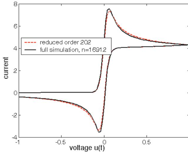
Fig. 4. Simulation results of the cyclic voltammogram when  $du/dt = \pm 0.5$ .
