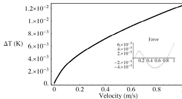
Fig. 6. Steady state solution for the temperature difference between the sensors for different flow velocities for the original and reduced models.
